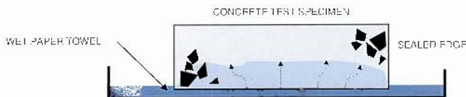
Figure 2.30: Water sorptivity test setup (Adapted from Alexander et al., 1999)
