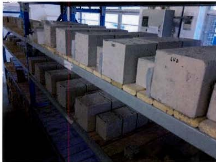
Figure 3.6: Simulated summer environment ( 53 \pm 2\% RH, 20 \pm 2\text{ }^\circ\text{C} )
