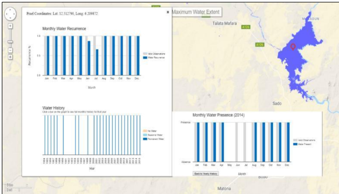
Figure 4-13: The monthly water recurrence, water history and monthly water history at Bakolori dam, while where data is not observed or masked due to cloud cover; the space is empty.
