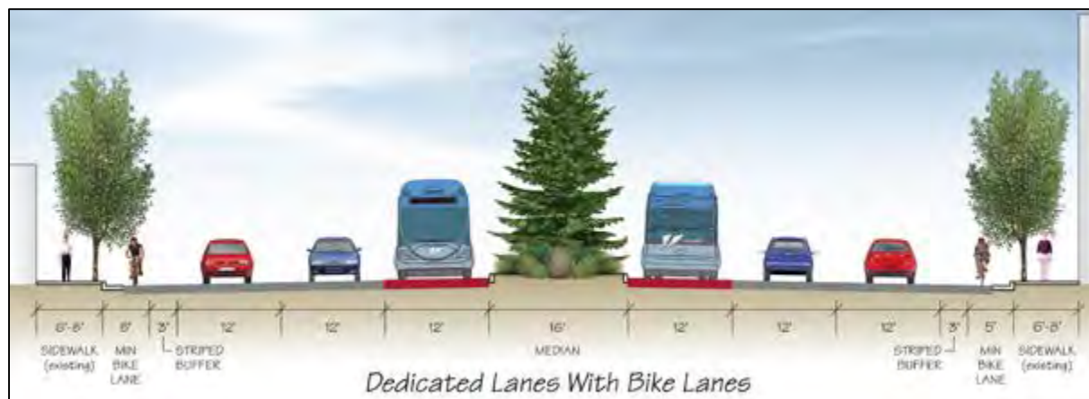
Figure 3-19 Median Busway Placement
