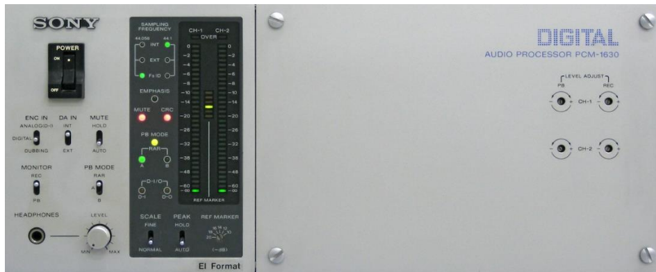
Figure 27. Van Gelder’s Sony PCM-1630 analog-to-digital. Source: (The Digital Era – RVG Legacy, n.d).
