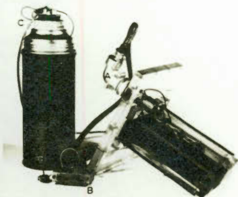
2. MODEL FITTED IN LID. NOTE SEAL WHERE THERMOCOUPLES PASS THROUGH. A=GOOSENECK TO SUPPORT WIRES. B=CANNON CONNECTOR. C=THERMOS FLASK WITH 0°C REFERENCE COUPLES.
