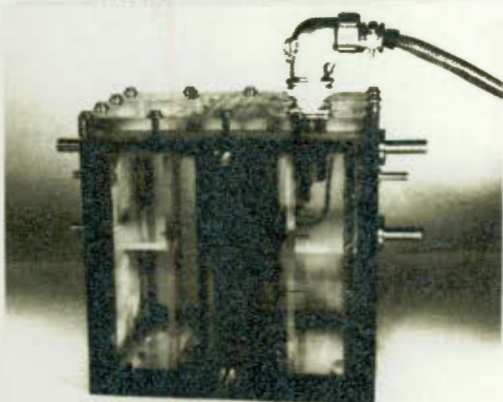
2. MODEL FITTED IN LID. NOTE SEAL WHERE THERMOCOUPLES PASS THROUGH. A=GOOSENECK TO SUPPORT WIRES. B=CANNON CONNECTOR. C=THERMOS FLASK WITH 0°C REFERENCE COUPLES.
