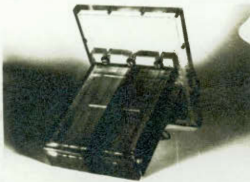
1. MODEL ASSEMBLED IN POSITION IN LID OF TANK. NOTE THE ADJUSTABLE CLAMPS WITH SEALS WHICH HOLD MODEL.
