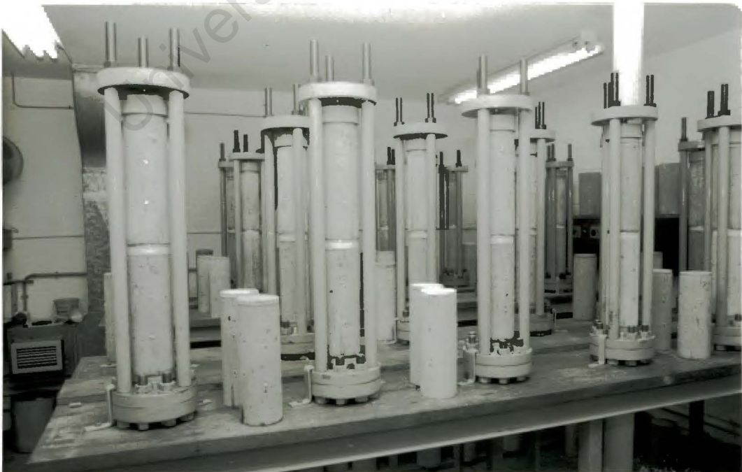
Fig.8.3. Each creep rig was loaded with two cylinders from two different mixes.
