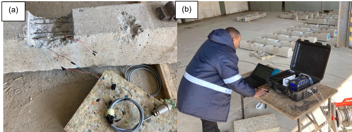
Figure 3.10: (a) Connectivity to the data acquisition system (b) Data acquisition system setup
