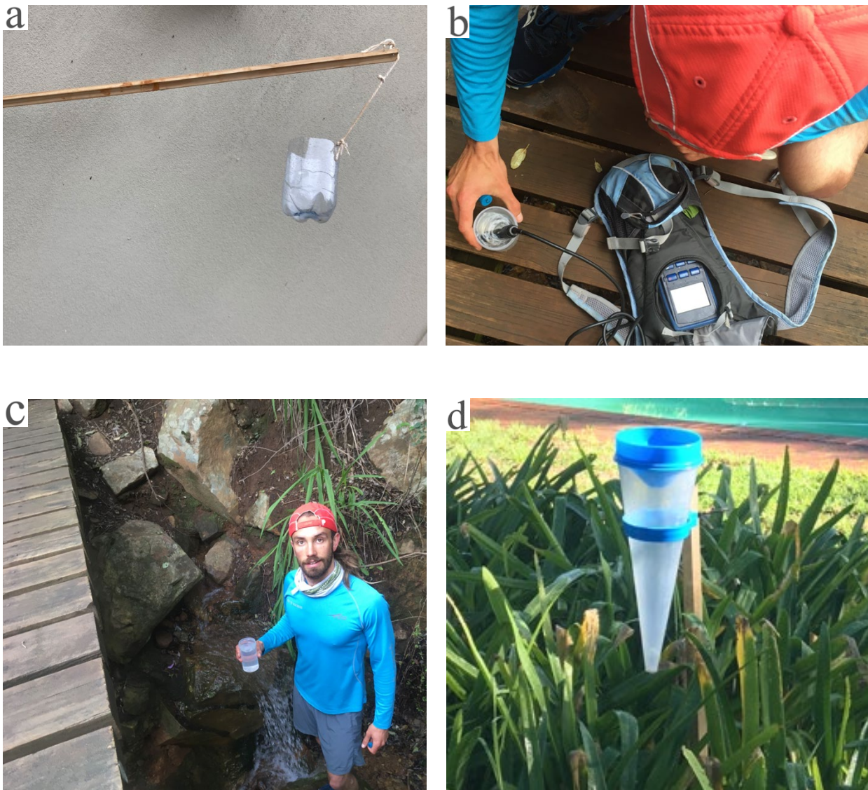
Fig 3.1 a Polyethylene terephthalate sample collection extension. b Infield electrical conductivity and temperature measurement. c Hout Bay stream sample collection. d rainwater collection in Hout Bay rain gauge.
