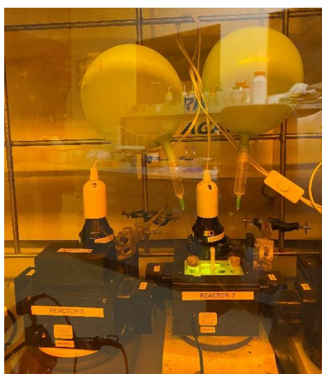
Figure 4.3. Typical set-up of the photocatalytic experiments performed in the EvoluChem™ PhotoRedOx Box.
