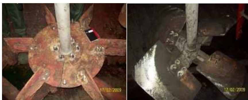
Figure 4 – Rushton and A315 Agitators used in the Secondary Leach Autoclaves
