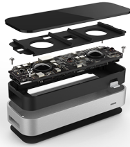
(a) Exploded view of the LMC [37]
