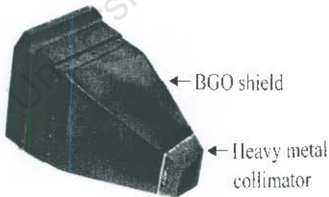
Figure 3.10: A BGO Compton suppression shield taken from [Duc99], showing the tapered heavy metal collimator (with a 35 mm by 35 mm entrance window for \gamma -rays) at the front end.
