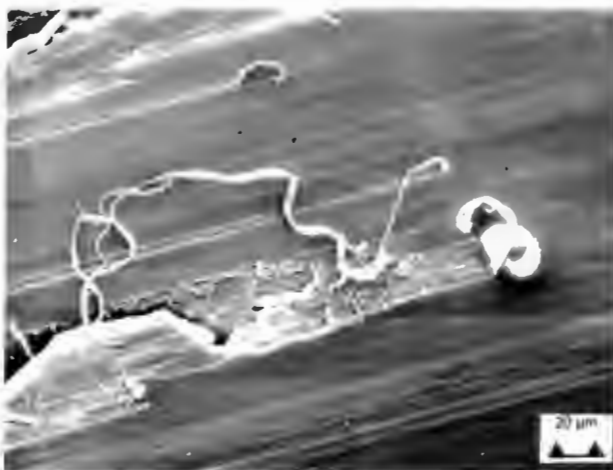
Figure 4.5 (f) UHMWPE pin run to 35 km in synovial fluid
