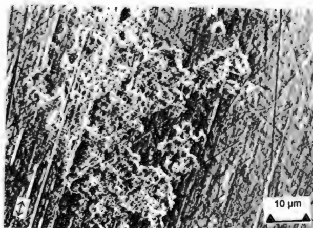
Figure 4.9 (III) Zirconia counterface run to 100km in distilled water
