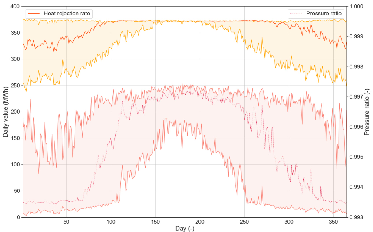
Figure 7-32: Intercooler daily cumulative heat rejection and pressure ratio ranges for a typical year
