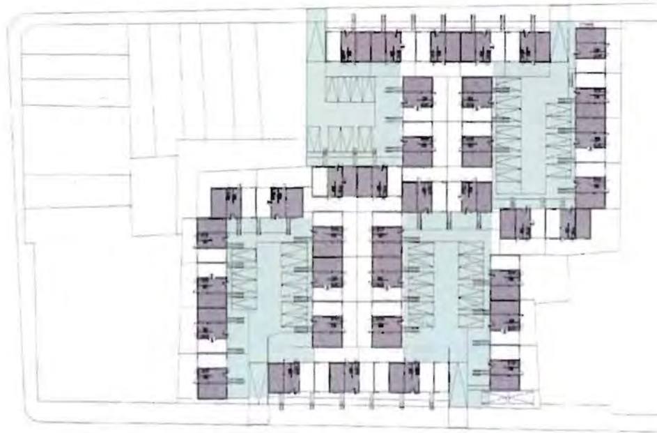
Above: Plan of the Quinta Monroy Housing Project illustrating the grouping of units around a collective public space. This condition introduces the idea of a social support structure through an ordering of shared public space (Lotus International 2011: 104)
