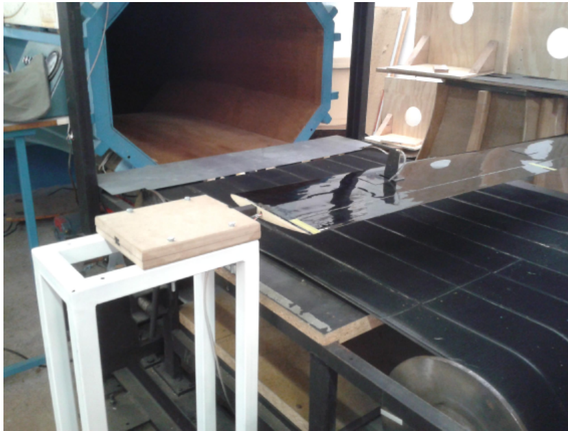
Figure 4.1: Photograph showing placement of the pitot tube on the wing. The photograph also show how the apparatus is positioned within the wind tunnel.
