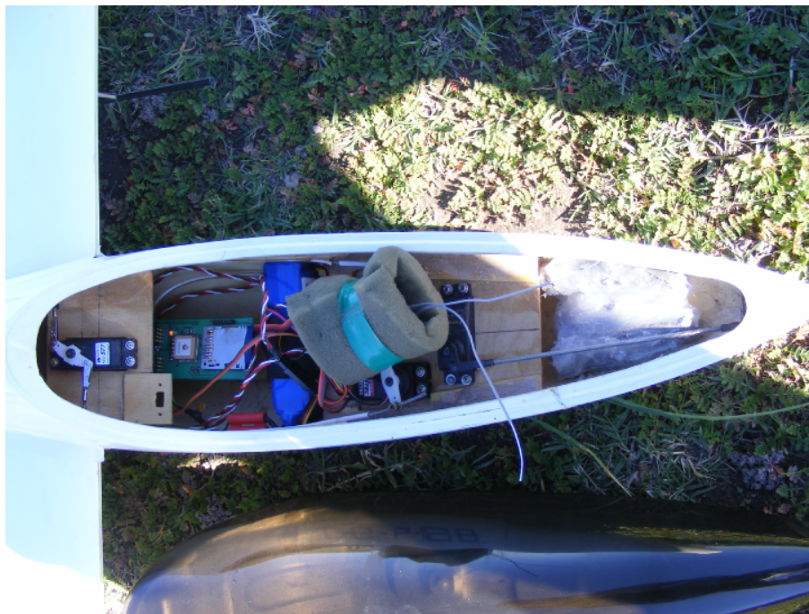
Figure 7.3: Photograph showing the placement of the device within the fuselage of the glider.
