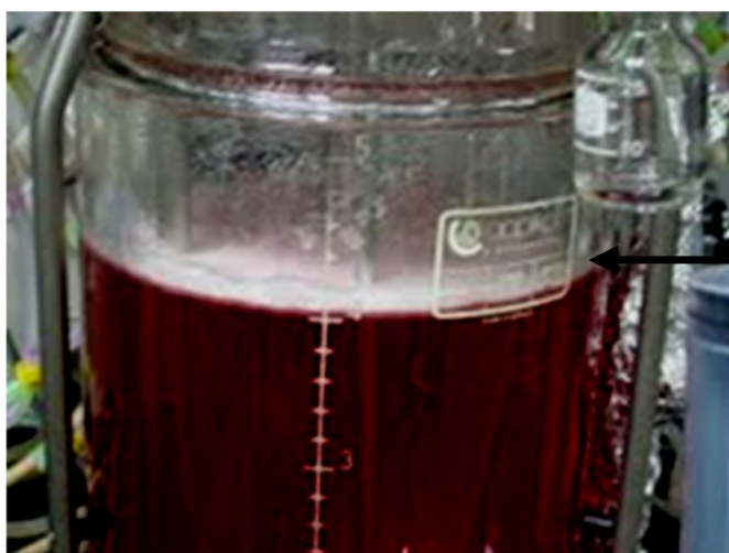
Figure 2-5 Effect of the foaming on microcarrier culture (Courtesy Panacea Biotec Ltd.)
