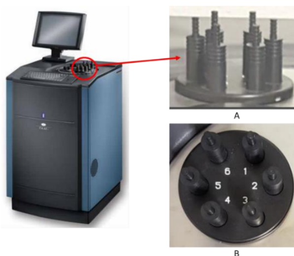
Figure 3-8 TAM III Isothermal Microcalorimeter (A) Side view of multichannel showed with red arrow (B) Top view of multichannel
