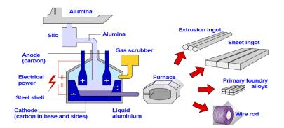
Figure 11: Aluminium production process
