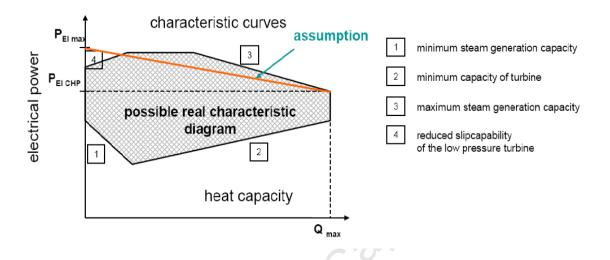
Figure 22: Heat to power relationship of a condensing steam turbine cogeneration system Source (Maurizio et al., 2008)
