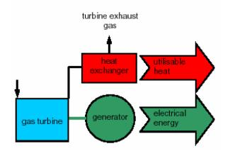
Figure 15: Simple cogeneration gas turbine configuration
