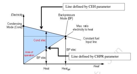
Figure 23: Heat to power relationship of a condensing steam turbine cogeneration system in TIMES Source (Maurizio et al., 2008)
