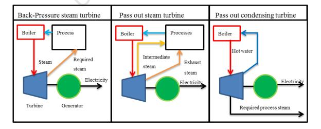
Figure 14: Steam turbine cogeneration systems
