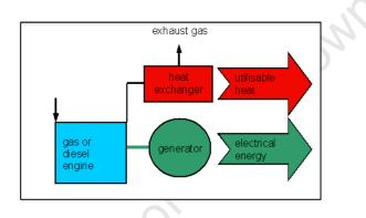
Figure 17: Internal combustion engine cogeneration system
