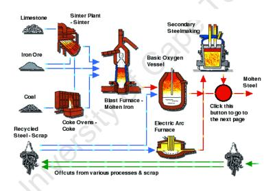
Figure 4: Conventional steel production process
