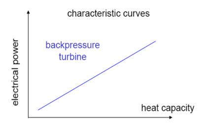
Figure 21: Heat to power relationship of a back pressure cogeneration system in TIMES
