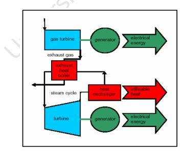
Figure 16: Combined cycle gas turbine cogeneration configuration Source: (Hernoe, 2004)
