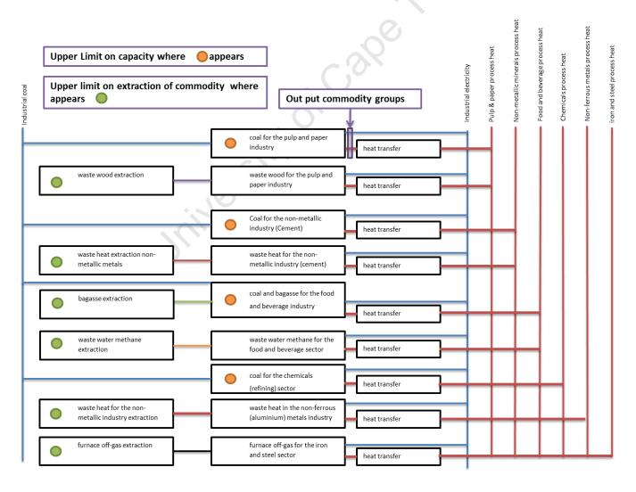
Figure 31: Reference energy diagram of cogeneration input into SATIM (2012)
