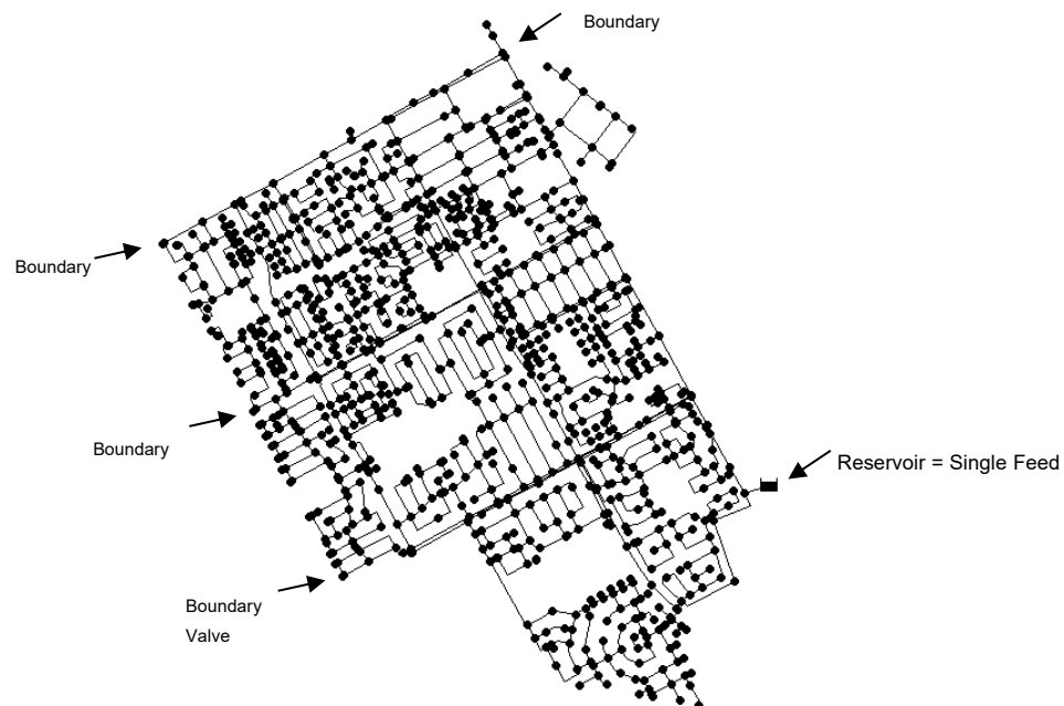
Figure 3-31: Snapshot of the Analysed Pressure Managed Zone Hydraulic Model. Extracted from Epanet
