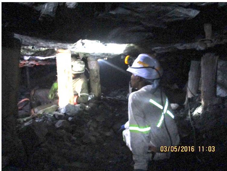
Photo 6: Miners working underground without masks.
