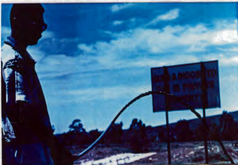
Plate 13: Borehole purging prior to sampling - borehole G40036, Gubb & Inggs. Note black colour of groundwater.
