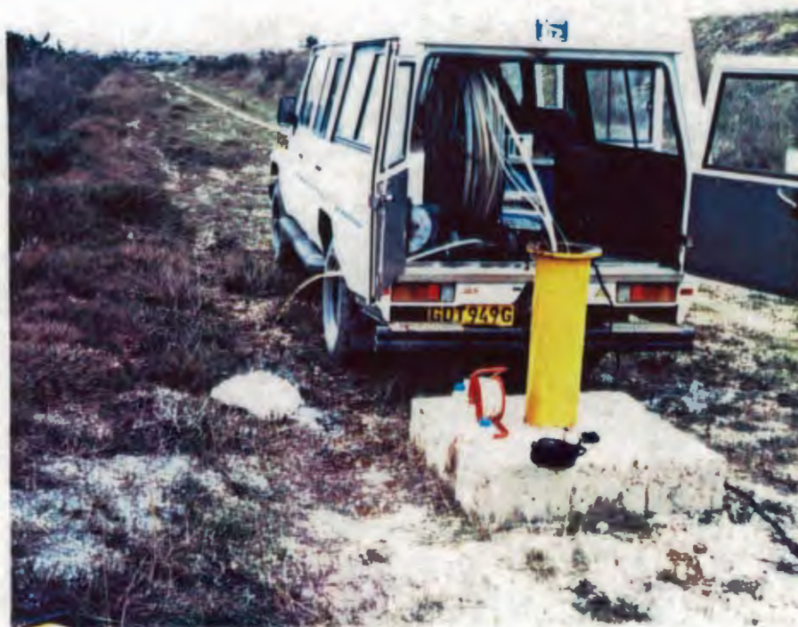
Plate 14: Borehole purging prior to sampling - borehole G40042, Cape of Good Hope. Note brown colour of groundwater and frothing on aeration.
