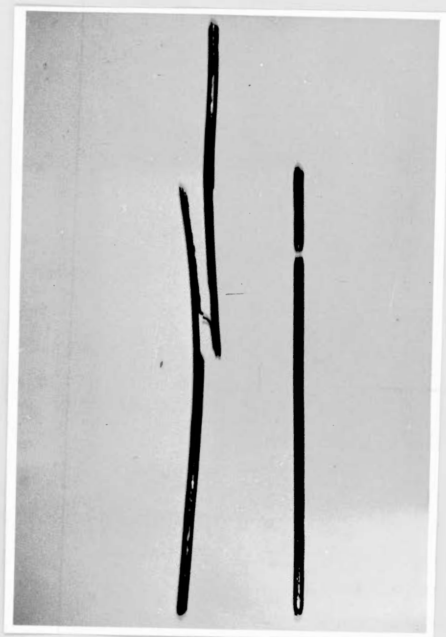
Figure 21c. Typical breaks in wires from sample 14. The wire on the left broke at 2400 lbs, the other at 3400 lbs. The first wire showed severe plastic deformation near the point of fracture.
