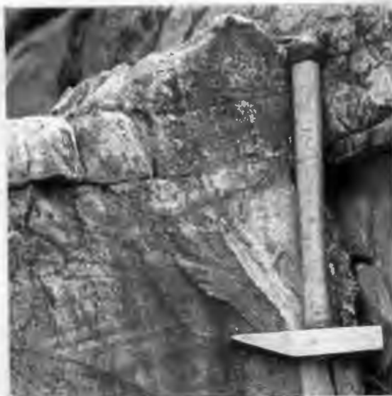
PLATE 2: Overturned trough cross-bedding in quartz-muscovite schist within the Pofadder Lineament (29°09'45"S/19°39'00"E).
