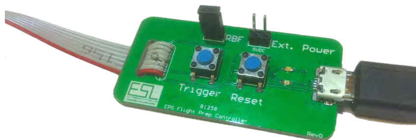
Figure B.1: Photograph of the Flight Preparation Controller interface.
