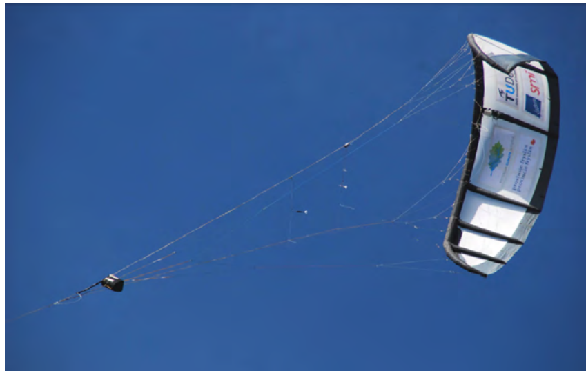
Figure 2.4.: KitePower's 25m 2 kite and control pod [4]
