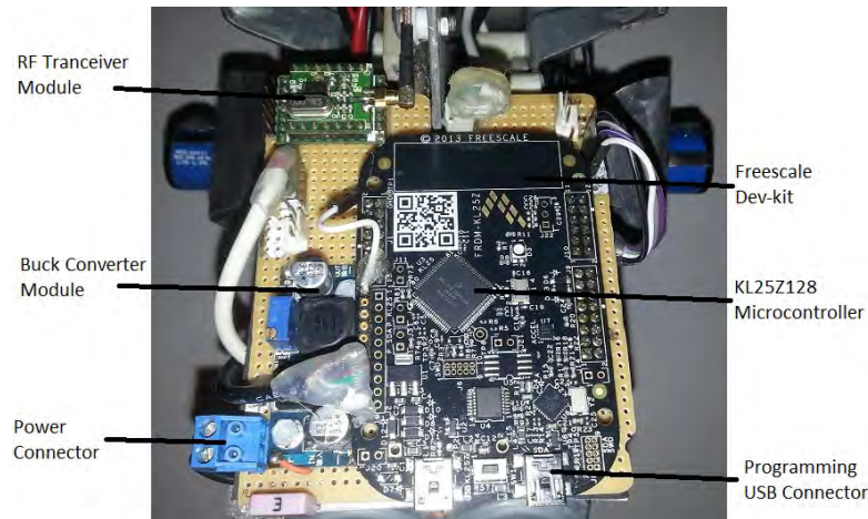
Figure 5.6.: Photograph of the system control circuit
