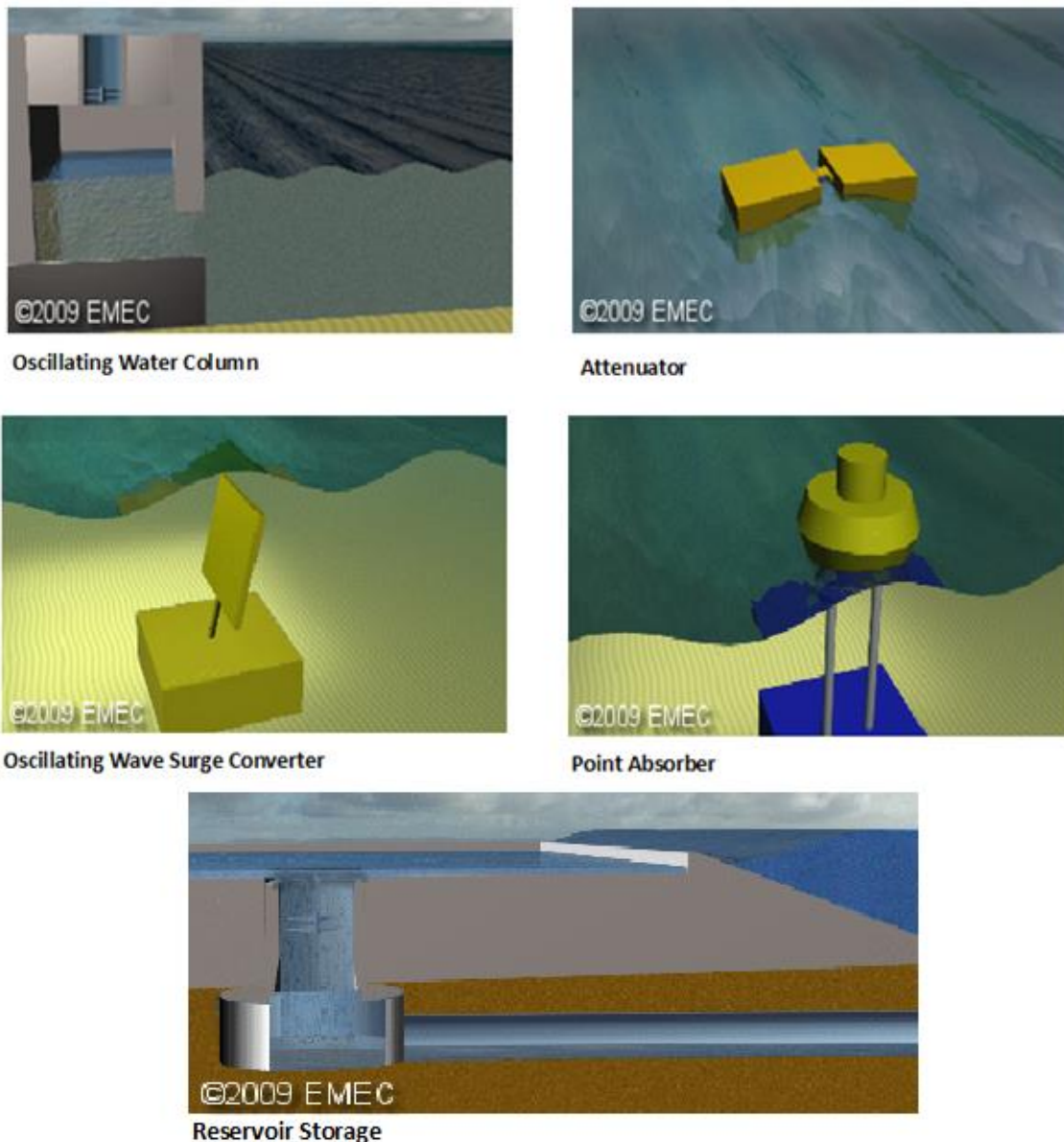
Figure 2-8: Operating Principles of Different Wave Energy Converter Designs (EMEC, 2012)
