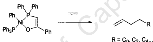
Fig. 1-2: A SHOP-type catalyst for the oligomerisation of ethene to linear 1-alkenes
