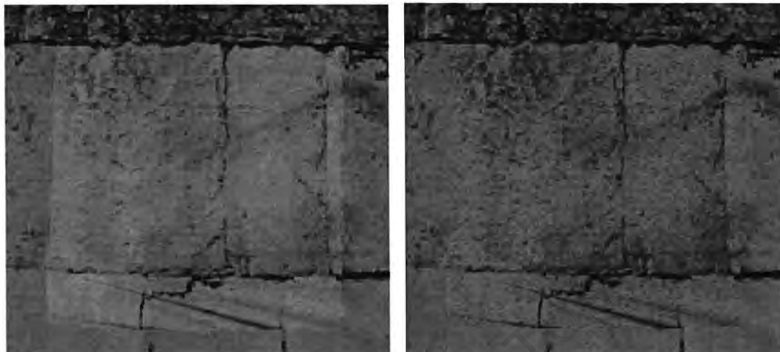
Figure 52 shows the use of the texture adjuster. The borders of the patch are far more visible with an unadjusted patch (a) than when the image is adjusted (b) by applying a 10% reduction in intensity.
