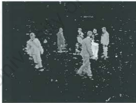
Figure 4.1: Segmentation using thresholded background subtraction.
