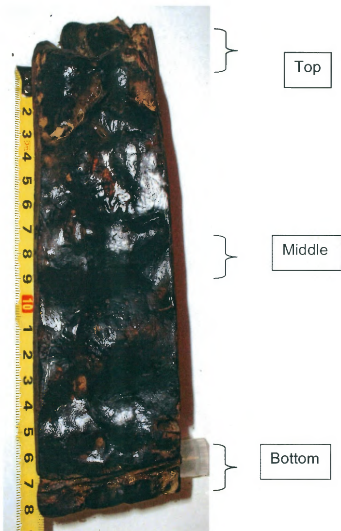
Figure 3.17 KB1-1 divided into three parts for radiocarbon dating.
