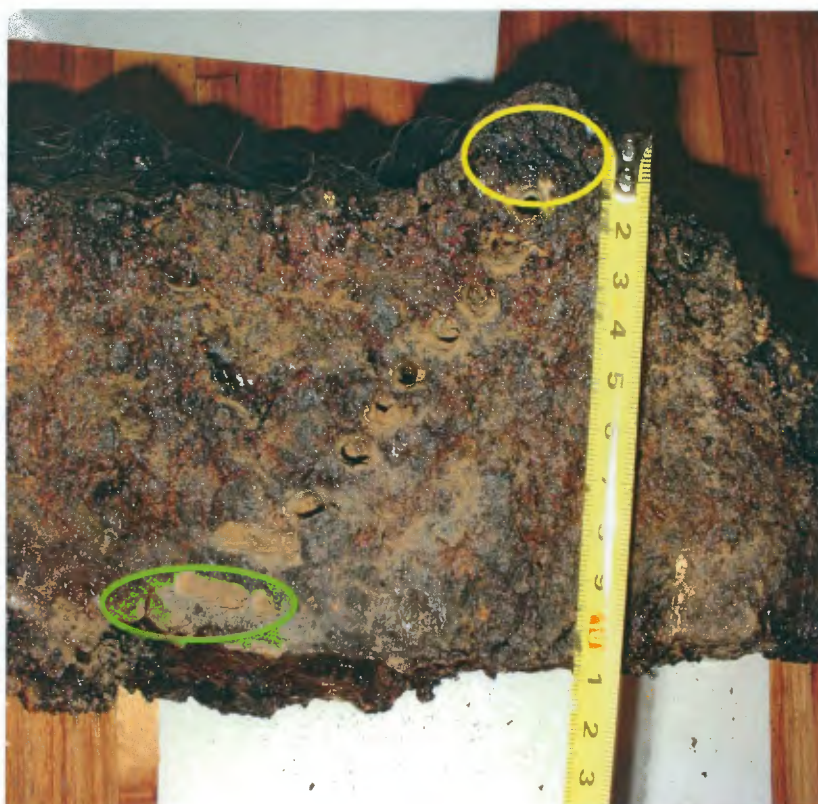
Figure 3.18 TK4 showing where the two samples for radiocarbon dating were taken.
