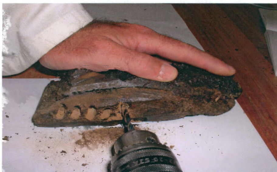
Figure 3.16 Drilling KB1-2 at intervals of about 1-2 cm.
