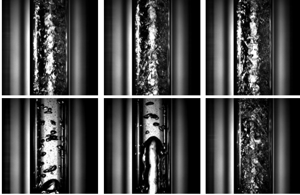
Figure 3.4- Flow Regime Misclassification by the Single Frame Model; Similar Annular images (Top row) are well classified, but more transient Slug-Churn images (Bottom row) are misclassified into Bubbly (Left), Slug (Centre) and Churn (Right) flows.
