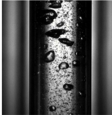
Figure 1.1- Two-phase flow; Gas bubbles are dispersed in a continuous upwardly flowing liquid phase.
