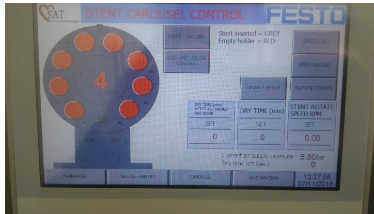
Figure 29 HMI used to program spray rig.
