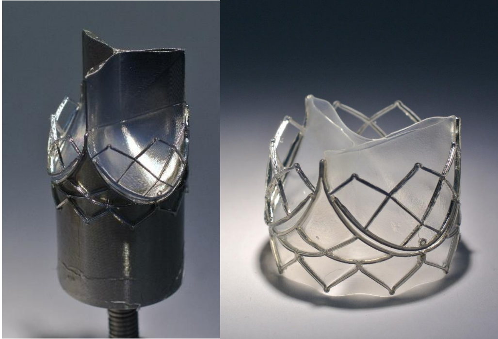
Figure 33 Valve before being removed from the mould (left) and valve after removal and free edge cutting (right).
