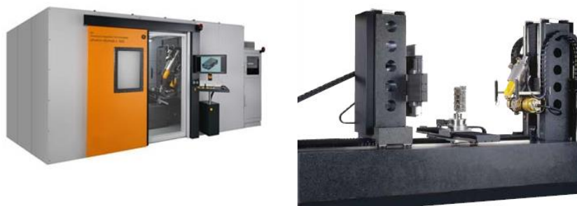
Figure 35 Micro CT scanner used for valve thickness analysis (Left). The valve was mounted and is rotated 360° while acquisition takes place (right).
