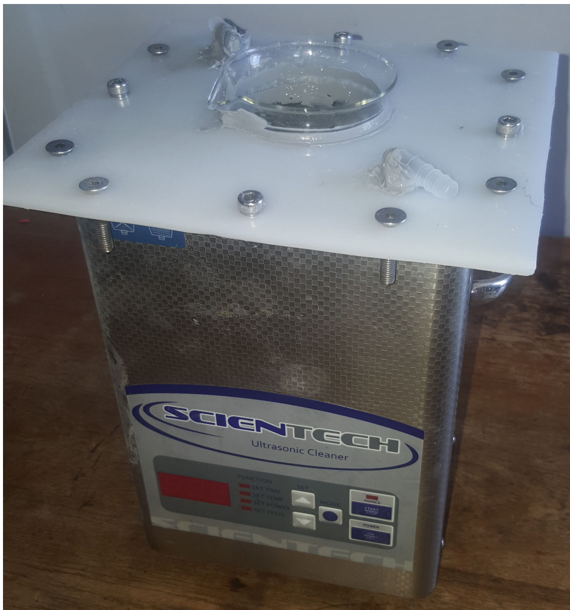
Figure D.2: Ultrasonic cleaner modified to create an internal jacketed beaker with coolant flow through the bath.
