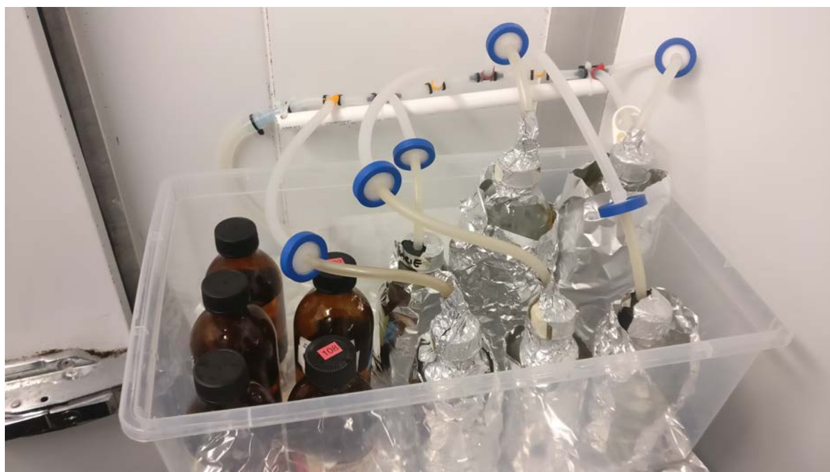
Figure 6.1: Experimental set-up for liquid incubation of melted spring cruise samples
