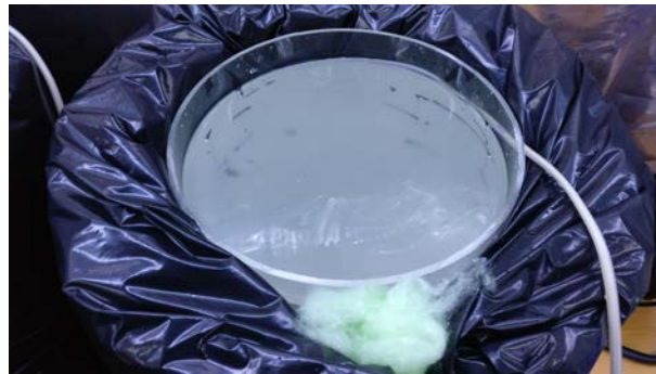
Figure C.5: Tank with closed insulation and heating cable
