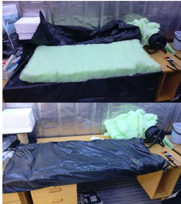
Figure C.2: Water- and forced convection proofing of Isotherm jacket
