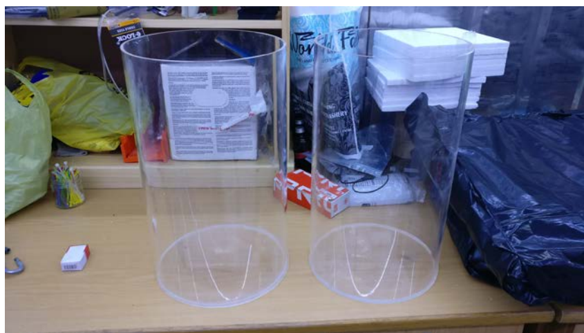
Figure C.1: Perspex tanks after bonding with bottom plates
