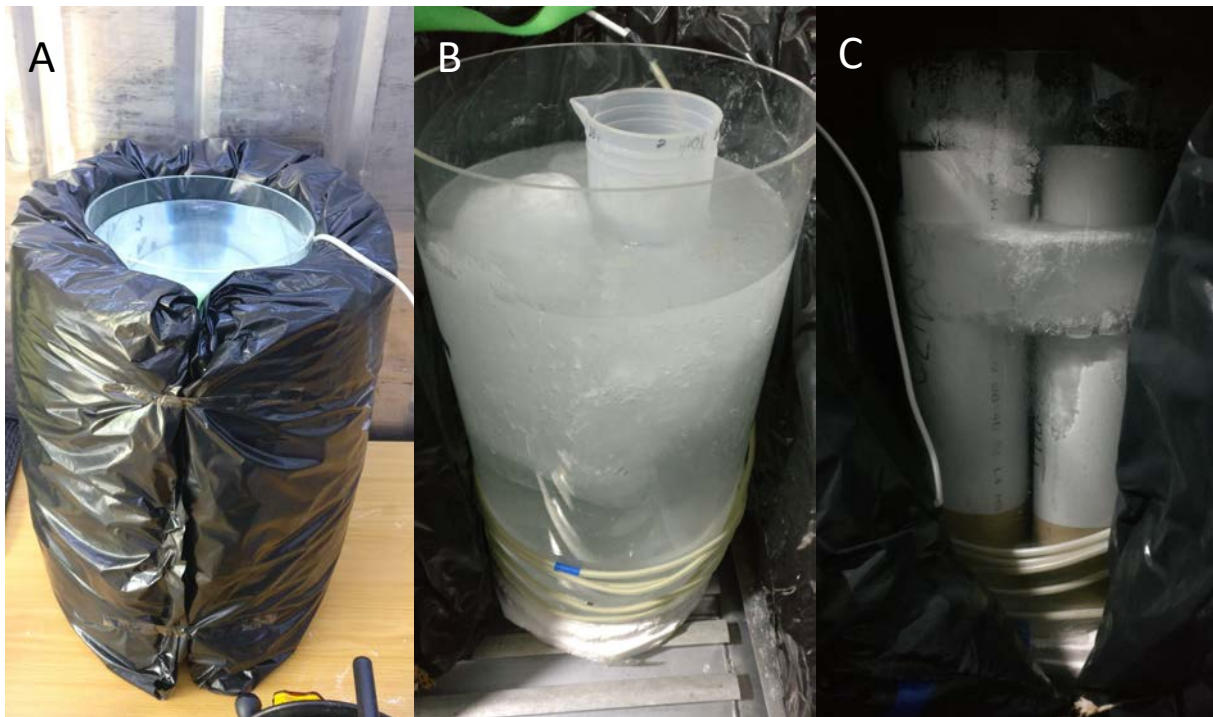
Figure C.6: Pictures of the hybrid system showing the (A) basic hybrid system with closed insulation (B) winter hybrid system with open insulation and (C) spring hybrid system with open insulation while lights are off.
