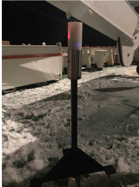
Figure 1.7: Novel ice drift, environmental monitoring and wave measurement autonomous platform: the Southern Hemisphere Antarctic Research Collaboration (SHARC) Buoy. Developed by the University of Cape Town. Photo by R. Verrinder.
