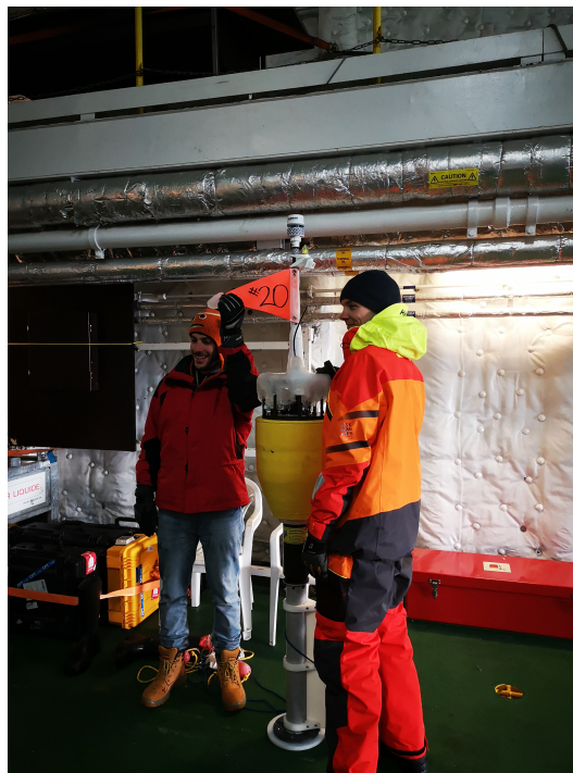
Figure 2.7: During the 2019 SCALE winter expedition, a SWIFT device was retrieved early due to lost communication with the host. This failure was attributed to a build up of ice along the rim from ocean spray. Photo taken by Author.
