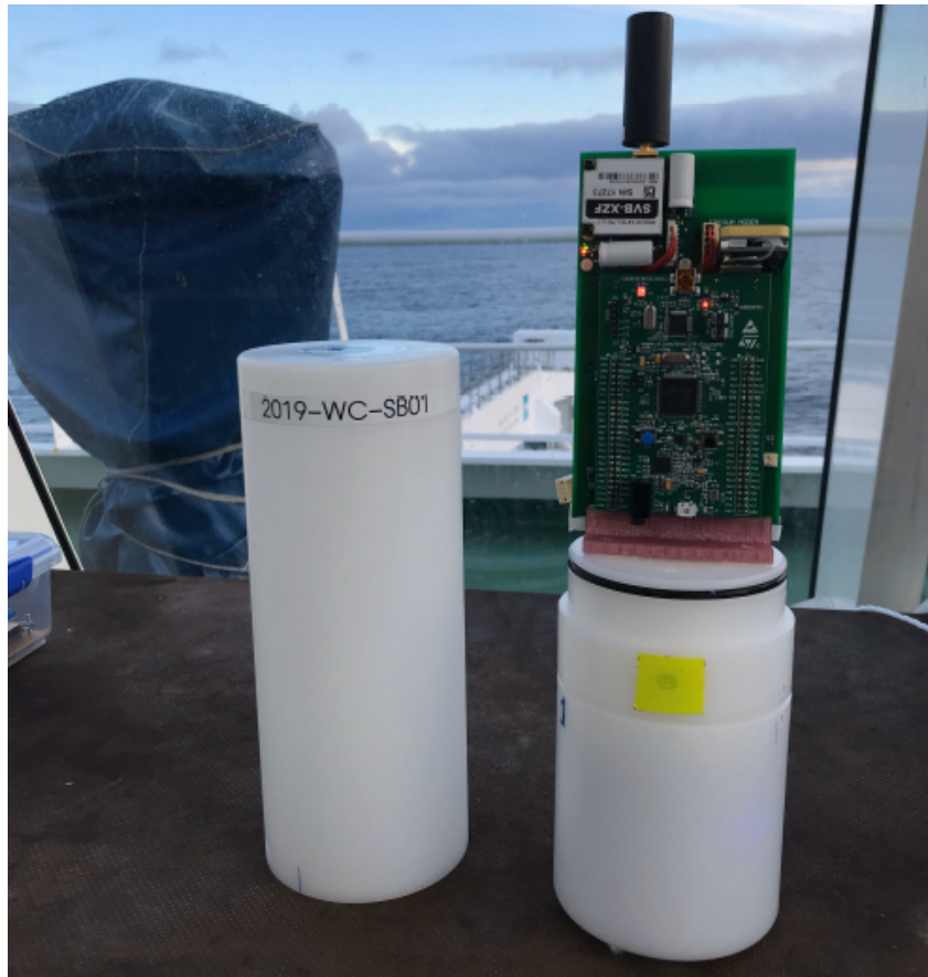
Figure 6.5: SHARC buoy version 1 used for deployment testing during the 2019 SCALE winter cruise in July. The device contains an Iridium modem, GPS and temperature sensor for sea ice drift and ambient temperature measurements. Photo by R. Verrinder.
