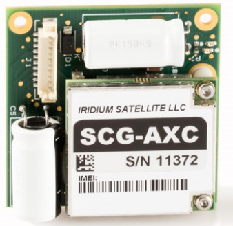
Figure 4.4: A Rock7 RockBLOCK 9603 satellite module containing an Iridium 9603 modem (Iridium Satellite Communications, 2019) and a coaxial Sub-miniature version A (SMA) connector for an external antenna. Image by Rock7 (2019).
