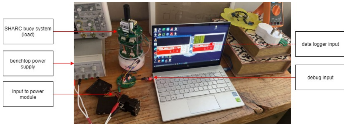
Figure 6.1: Diagram showing the configuration for the power test. All sub-systems were connected and activated with version 2 sensors and firmware. Power was supplied by an Agilent E3630A bench top power supply set to a constant 7.2 V output. A data logger was connected to the INA219 sensor to sample the power information at a rate of 1 Hz
