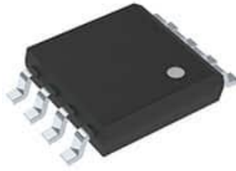
Figure 4.8: The Adesto Technologies SPI serial flash chips in a surface mount package. Image source: (Digi-Key, 2021).
