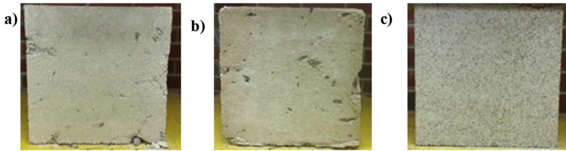
Figure 2-3: Triplicate rammed earth blocks after MICP treatment.
