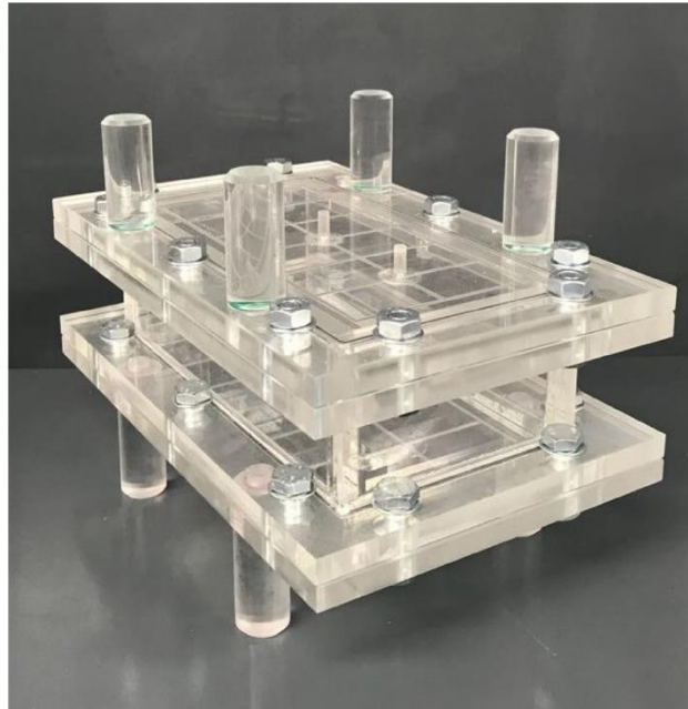
Figure 3-4: Picture of the Perspex bio-brick moulds. The bottom and top lids are identical and removable, both sealed with an O-Ring. To distribute the incoming liquid evenly over the sand body surface, the outside faces of both lids have three influent nozzles, and the inside faces have square depressions.
