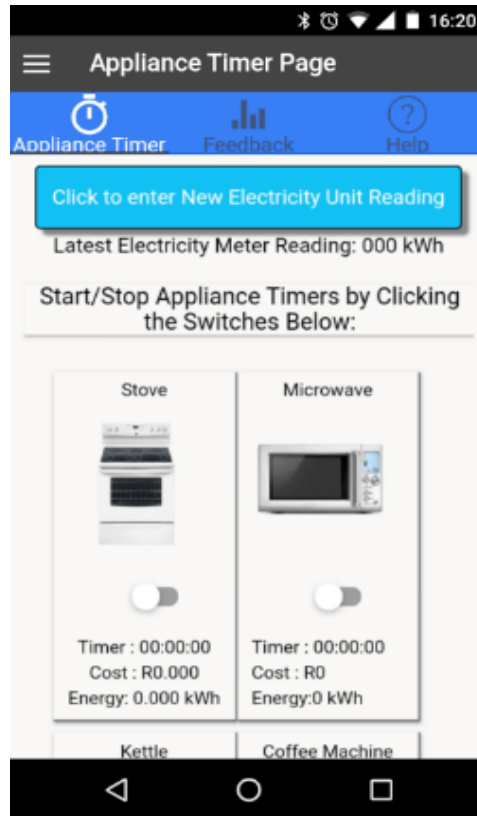
Figure 6: Screenshot showing the final user interface design for the mobile application
