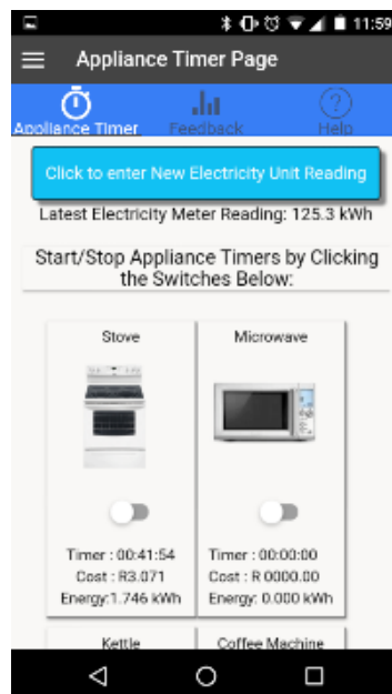
Figure 18: Mobile Screenshot showing the updated Appliance Timer tab once a new electricity meter reading has been captured
