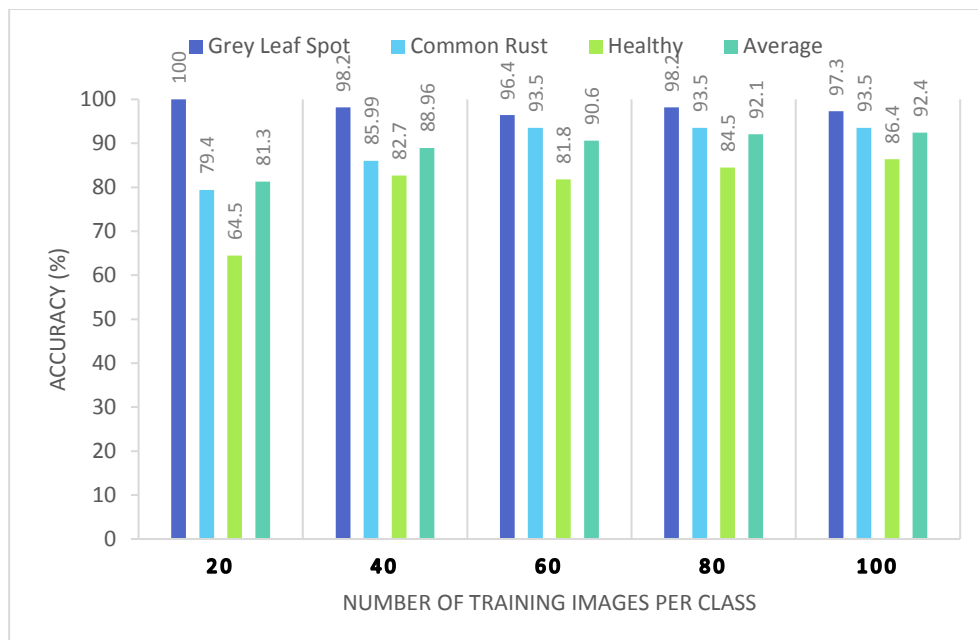
Figure 6-10 Effects of varying quantity of training data when training a SIFT-SVM classifier
