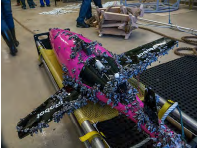
Figure 2.2 Glider covered in Goose-neck barnacles upon recovery from the Southern Ocean, highlighting the bio-fouling issues associated with long deployments.
