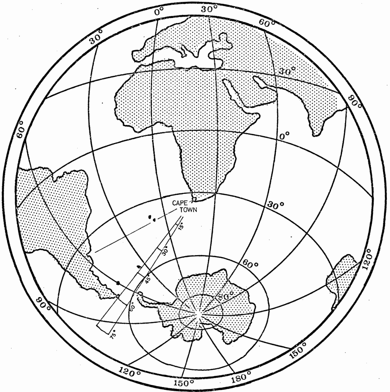
Fig. 2.9. Great circle paths to Cape Town as straight lines, with distances marked in terrestrial degrees ( 1^{\circ} = 60 \text{ n. m.} = 111 \text{ km} ).
