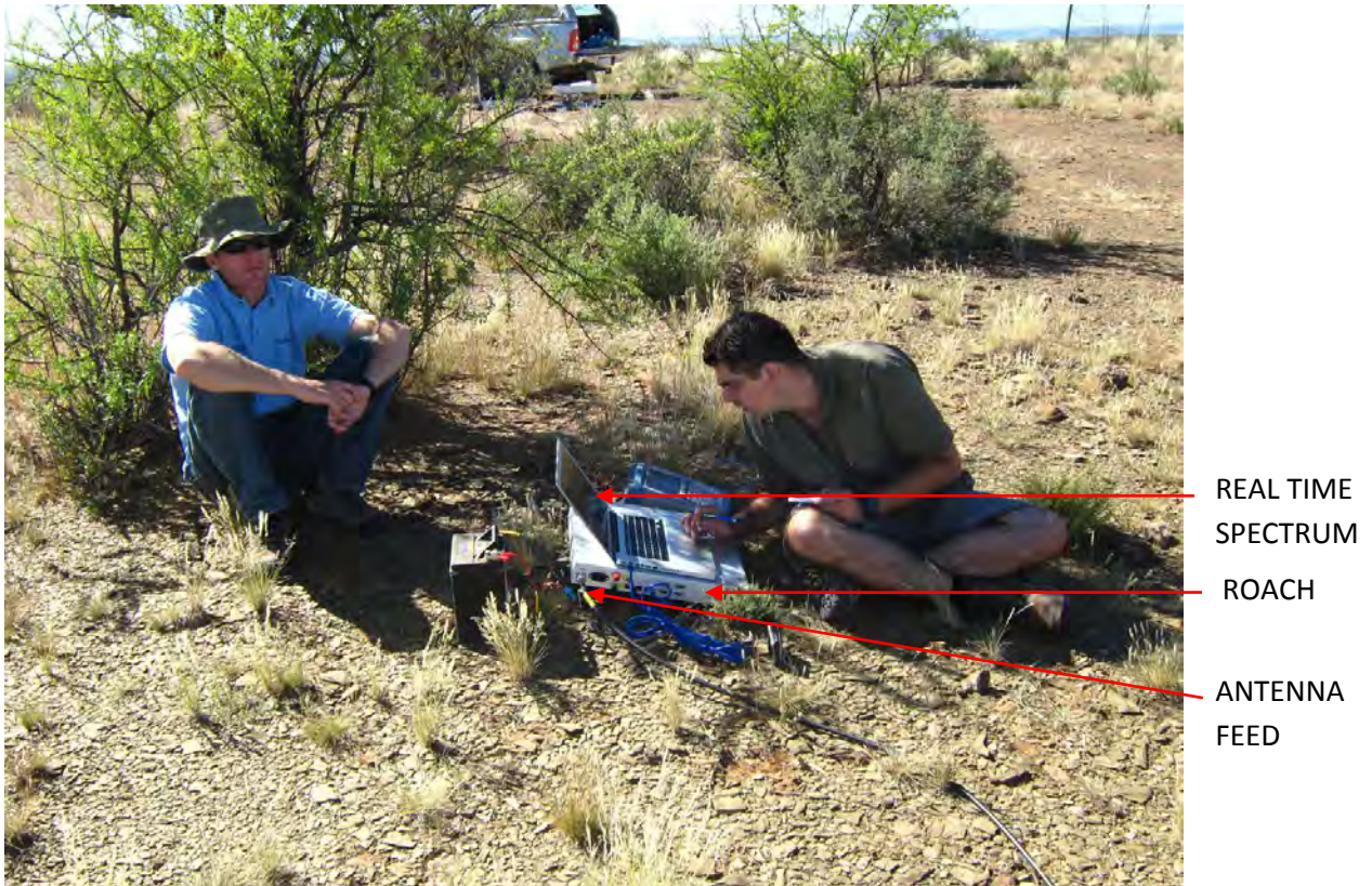
Figure 22 - Example of the RATTY system being used in the field
