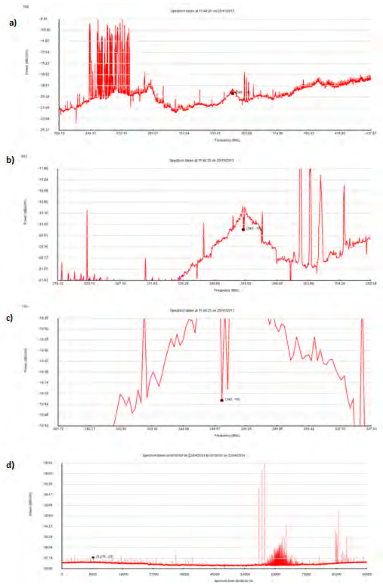
Figure 42 – a,b and c demonstrate the zoom function. Here we show progressive levels of zoom onto the black circle shown in a. As you can see it is simple to switch between a high level view and a very close view to see small scale details. d) Example plot of the channel 70.4MHz over 24 hours (86400 points). 70.4MHz is the frequency used by 2 way radio's on site.
