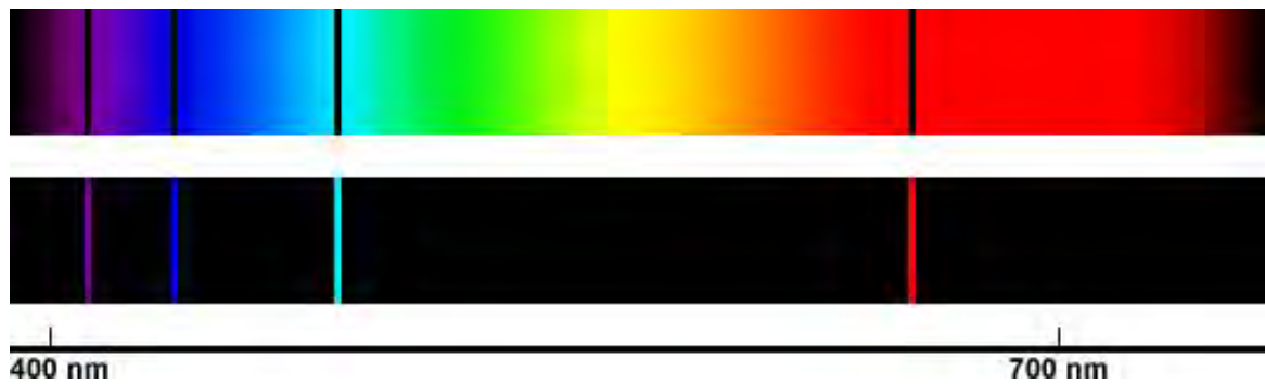
Figure 4 - Spectral lines of Hydrogen. The bar shows absorption lines and the bottom bar shows emission lines
