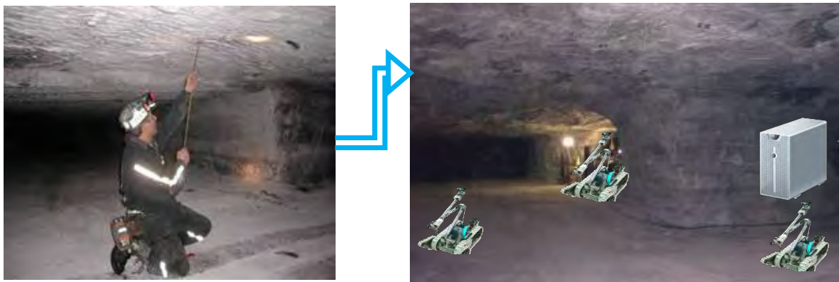
Figure 1.5: Overview of multi-robots supporting humans and performing cooperative inspection in an underground mine
