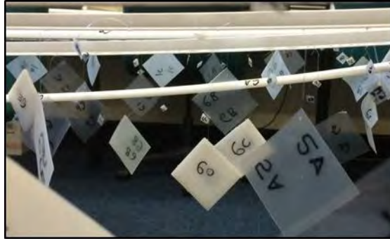
Figure 12: A selection of the samples tethered to the exposure rails before deployment
