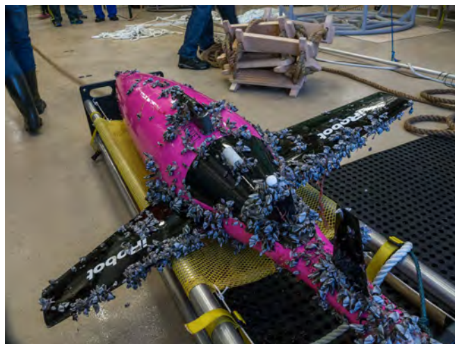
Figure 3.4: Goose-neck barnacles biofoul SG573 after 143 days at sea.
