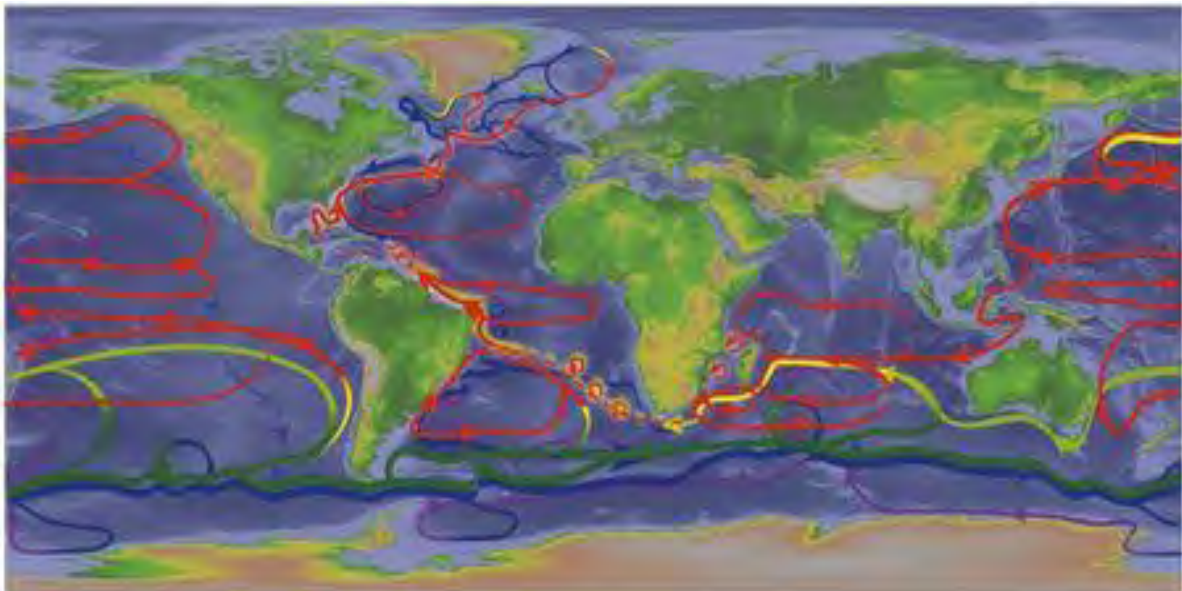
Figure 1: Schematic depicting the global Meridional Overturning Circulation. Red lines represent surface flows, yellow/ green represent intermediate flows and blue/ purple represent deep flows. (Base map by S.Speich adapted from Lumpkin & Speer, 2007 following Speich, et al., 2007)
