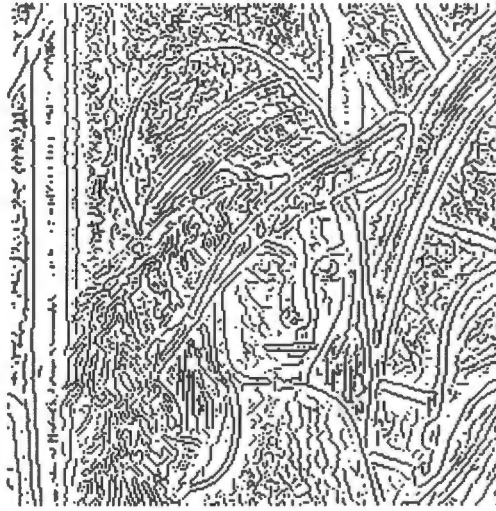
Figure 6.5: Edge point map. The edge points extracted from the second level of the wavelet decomposition, using the method of [33].
