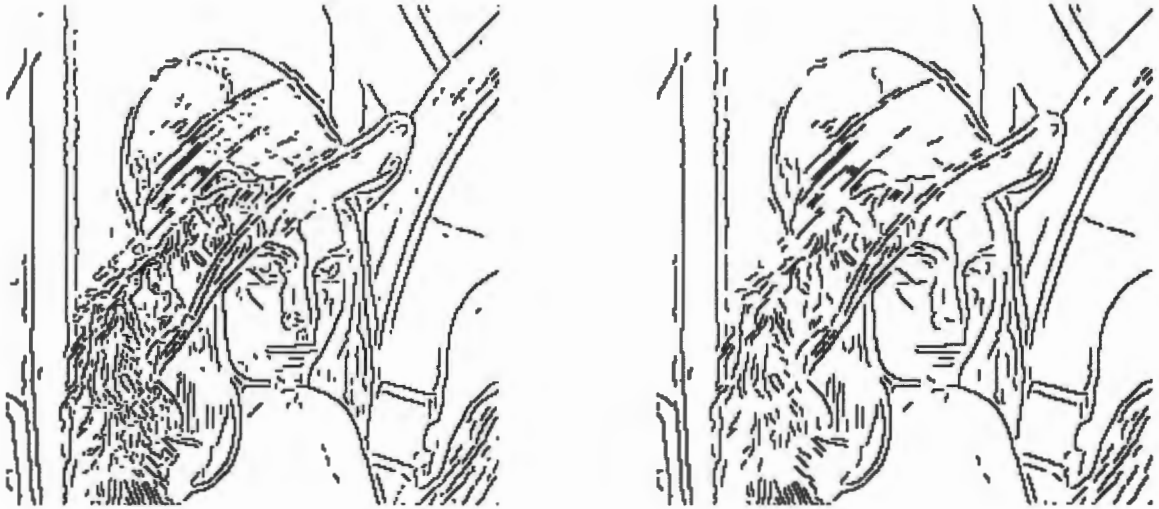
Figure 6.6: Extracted edge maps. The edge map on the left has 860 edges, while that on the right has 416. A edge length threshold was used for both — the left had all edges containing only one point removed. All edges with less than six edge points were removed from the second edge map.
