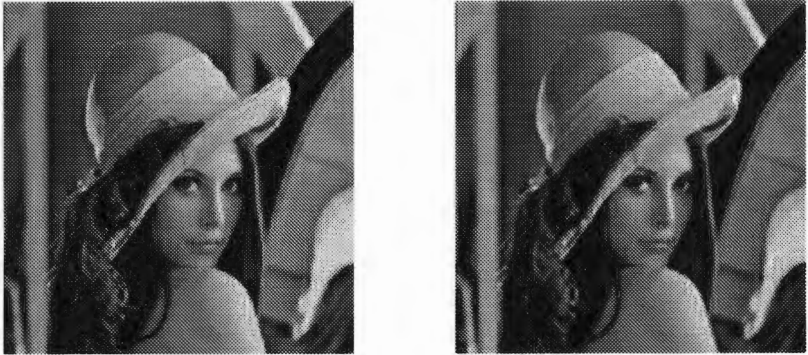
Figure 4.11: Typical compression results. The left image was compressed to 3.2:1 while the right image was compressed to 8.7:1. The maximum number of reproduction vectors for each sub-band was 256 (Figure 4.3) and no Huffman coding was used. The SNR's are 19.2 dB and 16.8 dB, respectively. Observe that quantization effects are immediately apparent as soon as a sub-band decomposition of two or more levels is used; in this example, both images exhibit these artifacts. The quantizers used were generated from the generic training set i.e., training set one.
