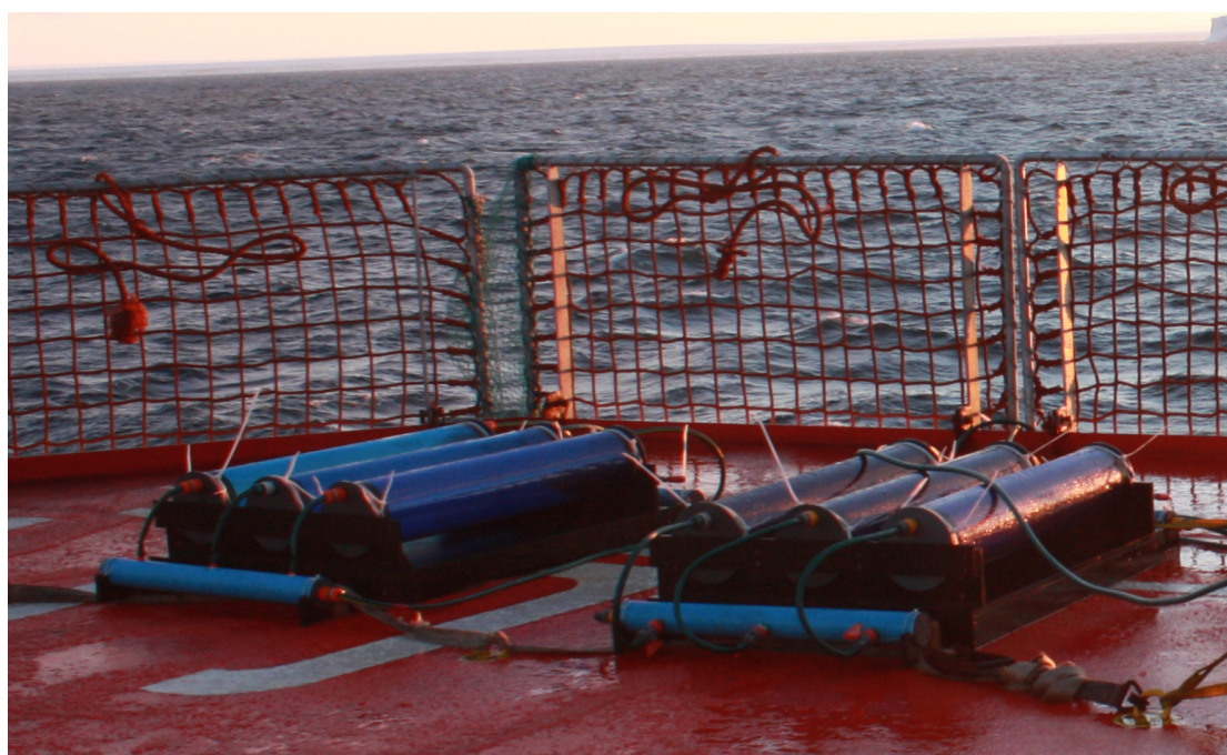
Figure 2.3.4 Photo of onboard primary production incubation set-up on the aft deck of the SA Agulhas . Tubes were covered in photographic filters to mimic the six light depths; from 54% to 1.1% (left to right) and cooled with a constant flow of surface seawater.
