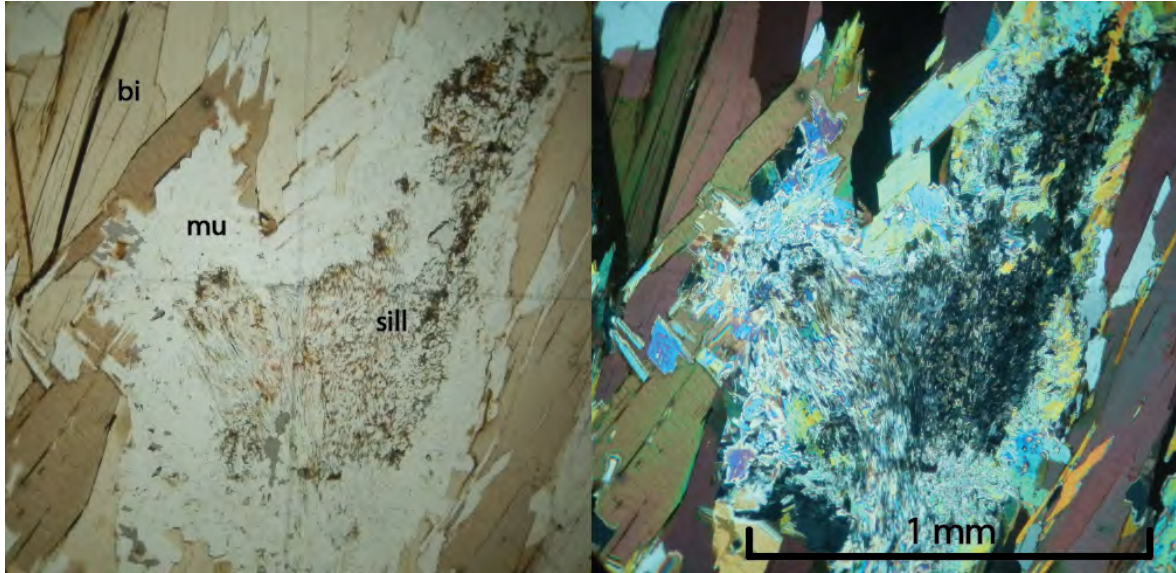
Figure 4.8: Thin-section textures in S64 showing a clot of sillimanite with a beard of muscovite, amongst coarser biotite.
