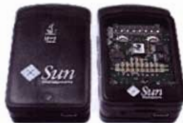
Figure 0. Sun SPOT (Small Programmable Object Technology). Left: a base station (or a transceiver); right: a sensor board
