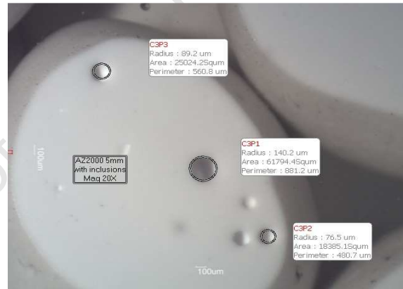
Figure 9: Air Inclusions in bead
