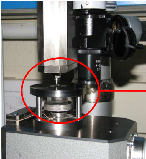
Figure 34: Test setup for ceramic bead friction coefficient measurement.
