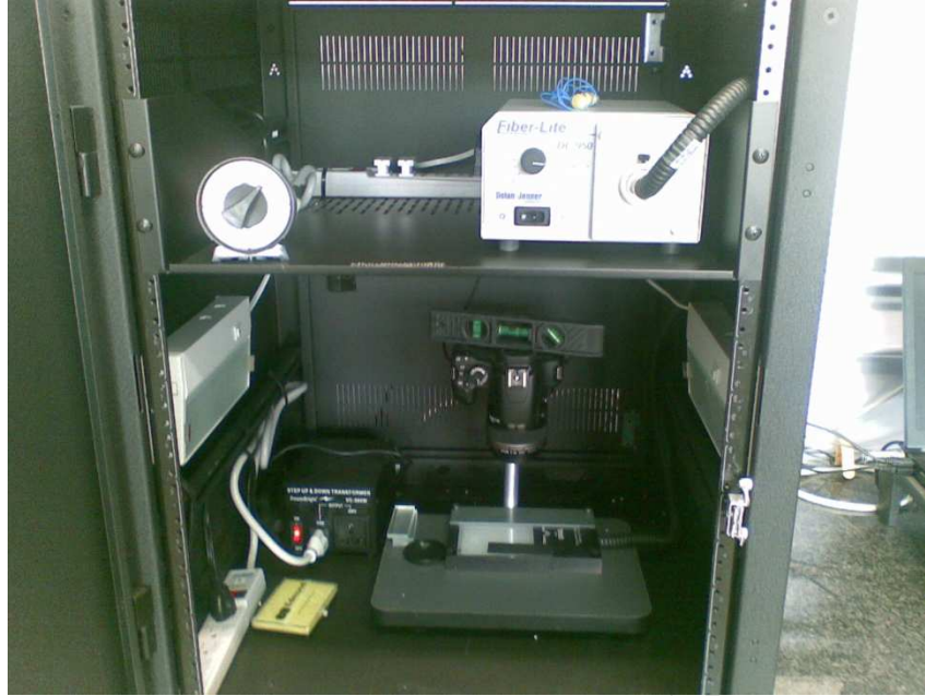
Figure 38: Custom Built Ceramic Media Sizing Equipment
